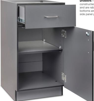
**Drawers -** Full height drawer sides are constructed with 1/2" thick phenolic resin and are rabbeted and screwed. Drawer bottoms are 1/4" phenolic resin trapped into side panel grooves.
