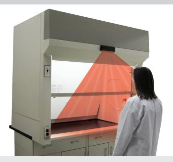
**Overhead Presence Sensor** – When a user leaves the hood unattended, the sash automatically closes after a pre-set amount of time determined by the user (30 seconds to 30 minutes). When the sash is closed, other workers are protected from the contents of the fume hood.
